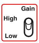
This 2 positions switch allows you to select the desired gain on the output.
