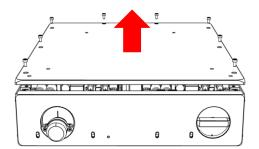
Remove the eight screws from the top panel of the Nagra CLASSIC PHONO with the supplied Allen key (2.5 mm). Then vertically lift up the top panel to open the device.
