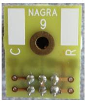
Each load circuit is numbered and matches precise load values:
