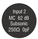
Figure 5: Configuration for moving coil cartridge with subsonic filter engaged.
