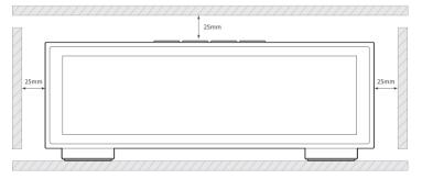
• Secure a depth of 35 cm for airflow and cabling.
