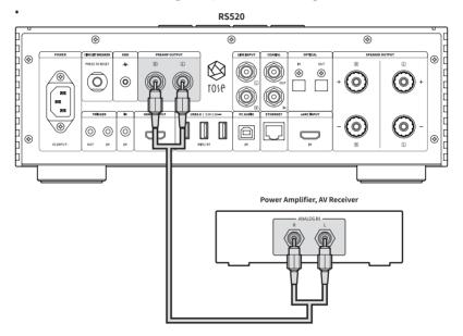
▲ **Caution:** Before connecting this product to a power amplifier, set the volume of this product to mute or to level 5 or lower and then connect using an RCA cable. If the product is playing music and the volume is turned up, a loud shock sound may be produced when the cable is connected.
