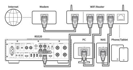
\* To control this product from the mobile application (ROSE Connect Premium), the product and smartphone must be connected to the same network. (You can configure one network by using a wireless network extender, bridge, etc.)
