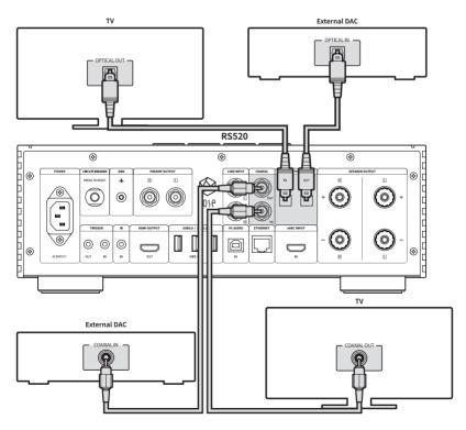
▲ **Caution:** Do not input signals other than linear PCM signals such as Dolby Digital, DTS, AAC, etc. to this device. Otherwise, noise may be generated and the speaker may be damaged.
