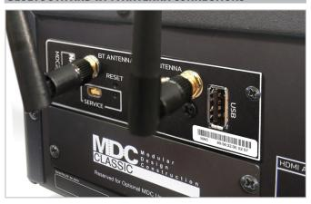
Connect supplied Bluetooth antenna and Wi-Fi antenna\*
