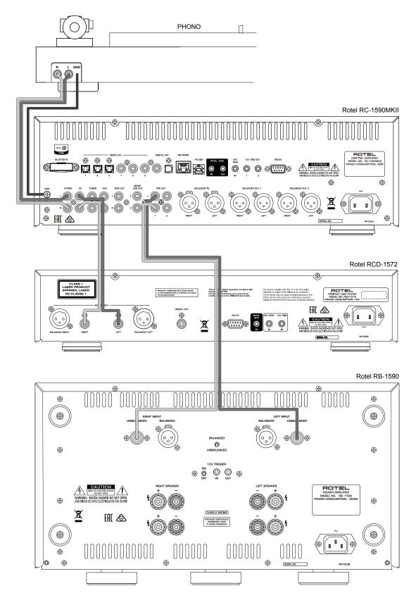
Figure 4: Balanced (XLR) Input and Output Connections
