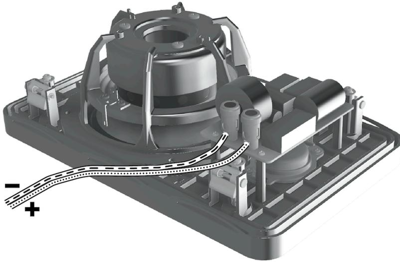
With the Speaker Unit connected to the speaker cable it can be inserted into the Installation Frame. Turn the locking tabs on the front surface of the Speaker Unit fully clockwise (aligned with the lock icons) and insert it in the Installation Frame. Push gently around each locking tab until a click is heard. The Speaker Unit will then be secured in the frame.
