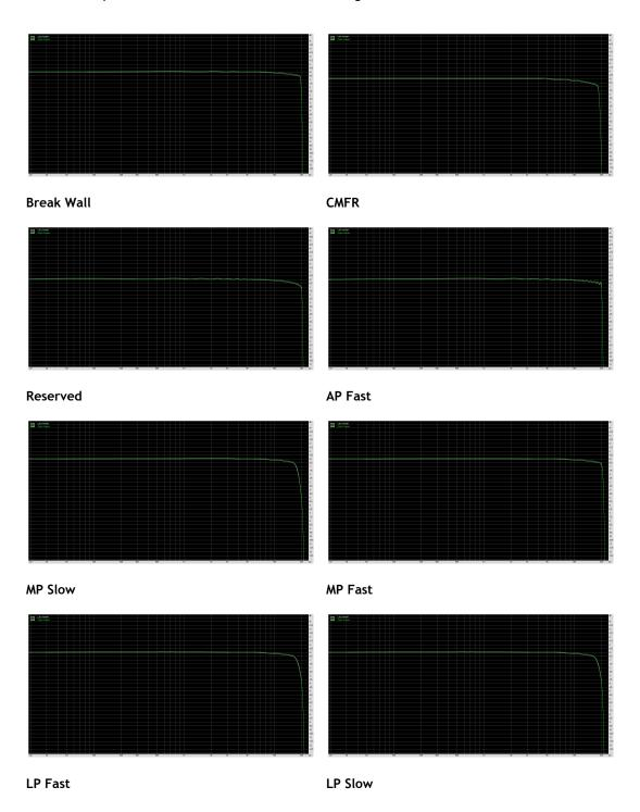
FIR Filters are part of the digital process built in the DAC chip. These filter settings mainly affect high-frequency roll-offs usually in the 18khz and above frequency range. The effect of the filter settings is very subtle and may not always be audible.
