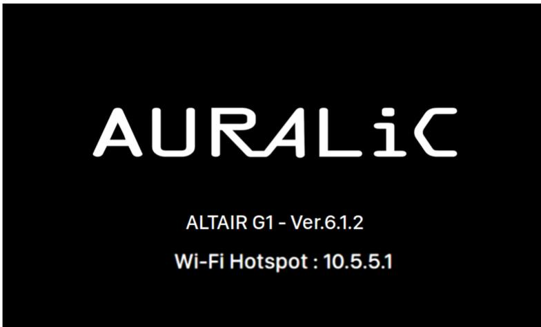
'Wi-Fi Hotspot' indicates that the ALTAIR G1 is broadcasting a Wi-Fi signal used for setting up the device on your home network. Make sure you have plugged a network Ethernet cable into the back of the ALTAIR G1.
