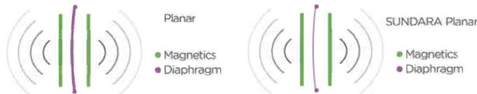
Compared to conventional dynamic driven headphones, planar magnetic headphones have solved problems such as surface distortion of high frequency audio and the lingering vibrations in a dynamic loudspeaker. The large and heavy magnets used face a residual vibration due to the retained momentum in the driver as it moves. In a Planar Magnetic the utilization efficiency has been improved by the weight of drivers being reduced with the use of our ultra-fine diaphragm in the SUNDARA.
